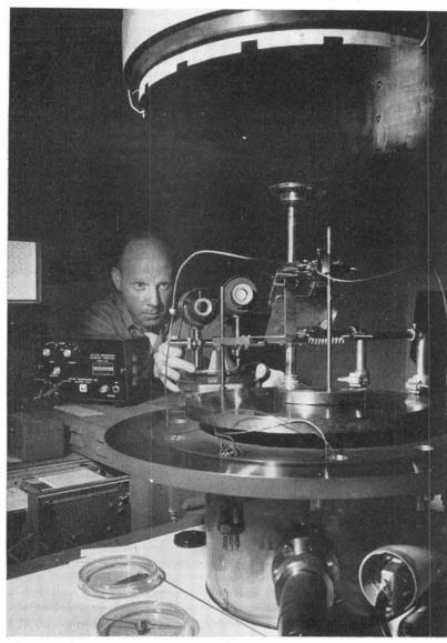
L. E. TERRY (1433) adjusts optical thickness monitoring equipment to prepare for vacuum evaporation of silicon monoxide insulating films. The Section is developing thin film devices to use with thin film circuitry.
